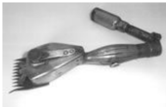
A 'Wolseley' mechanical shear
